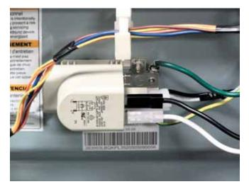
4. Remove the 2 (7-mm) hex-head screws that hold the filter to the frame.
