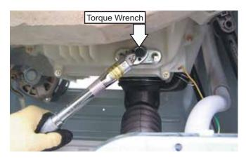
**CAUTION:** Proper torque must be applied to the 10mm hex nut to assure a proper seal. Under torquing could cause water leakage; over torquing could cause the tub to crack.
