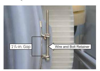
5. Pull the tub gasket off the outer tub lip.
