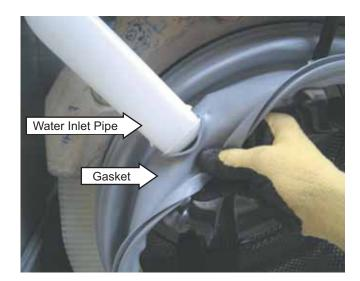
4. Loosen the 7-mm bolt that holds the wire and bolt assembly to the outer tub lip. Remove the wire and bolt assembly from the tub gasket.
