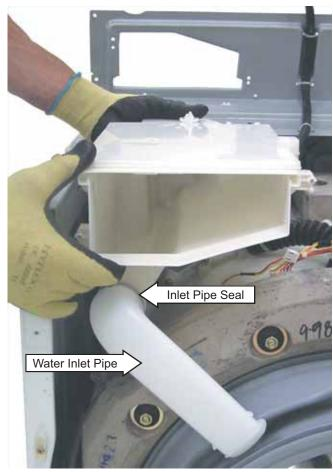
**Note:** The inlet pipe seal is difficult to install, place a small amount of liquid soap on the seal. Install the inlet pipe in alignment with the indentation at the bottom of the dispenser tank.
