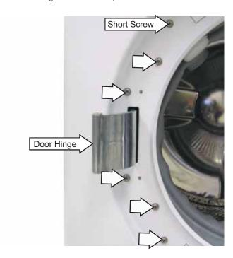
Caution: When reinstalling the door hinge, be sure to use the short screw on the top. Damage to the dispenser inlet may result if the wrong screw length is used.
