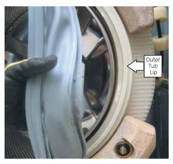
**Note:** When reinstalling the tub gasket on the outer tub, align the notch in the gasket with the arrow located on the top of the outer tub lip before tightening the wire and bolt assembly.
