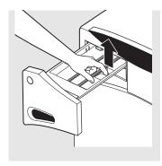
■ Remove the inserts from the bleach and fabric softener compartments and the detergent insert. Rinse the inserts and the drawer with hot water to remove traces of accumulated laundry products.
