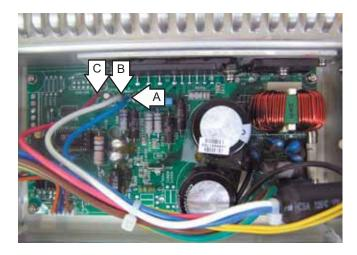
**Note:** The sensor and sensor wiring can be checked at the control board. Check for a resistance value of approximately 118  $\Omega$  resistance between the 2 yellow wires located on the wire harness located at P9.
