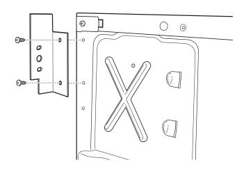
5. Align the holes in the right bracket with the holes in the bottom right corner of the dryer. Attach the bracket using 2 (#12 x 1-in.) Phillips-head screws.
