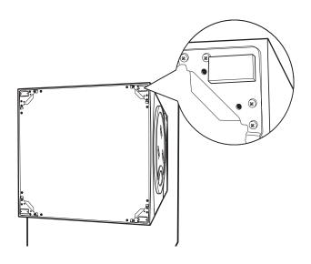
4. Align the holes in the left bracket with the holes in the bottom left corner of the dryer. Attach the bracket using 2 (#12  $\times$  1-in.) Phillips-head screws.
