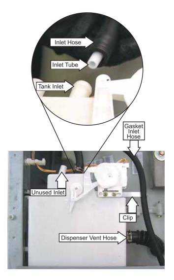
**Note:** Reinstall dispenser vent hose with notch aligned on dispenser tank and ensure seam remains aligned with the pointer on the outer tub.
