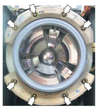
10. Remove the counterweights and the 8 bolts from the slots in the outer tub.
