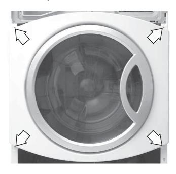
7. Lift up then remove the front panel from the 2 hooks.
