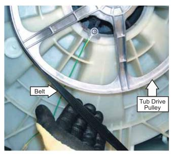
**Note:** The belt is elastic and is designed to be removed and installed in this manner.
