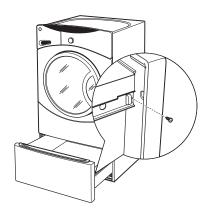
19. Remove the 4 shipping screws from the back of the washer.
