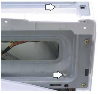
8. Remove the 2 Phillips-head screws that hold the dispenser to the front bracket.
