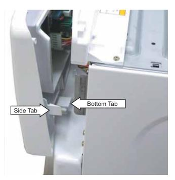
6. Lift the top edge of the panel to disengage the 3 tabs that hold the top of the panel in place.
