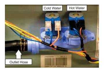
4. Remove the single (6-mm) hex-head screw that holds the valve to the cabinet.
