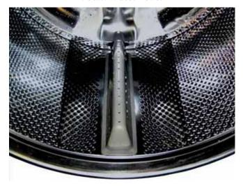
The main water level is approximately  $1\frac{1}{2}$  inches below the door opening and approximately  $2\frac{1}{8}$  inches deep at the bottom center of the wash basket.
