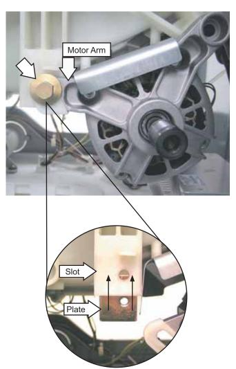
**Note:** The threaded plate can fall out of the recessed slot in the motor mount. Ensure this plate is reinserted in the slot upon reassembly.
