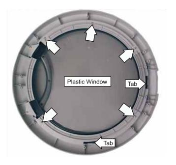
8. Slide the protect cover and ring away from the handle side of the door frame.
