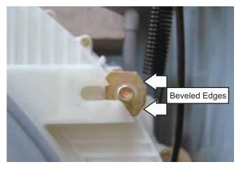
**Note:** To make installation of the front bottom counterweight easier, secure the placement of the bottom bolts with electrical tape.
