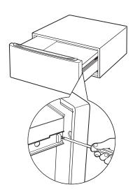
**Note:** The support pads should be installed on the dryer only. **DO NOT INSTALL THE PADS ON THE WASHER PEDESTAL.**
