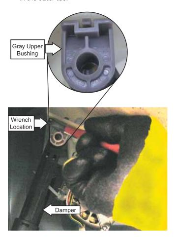
3. Remove the pin that secures each damper to the chassis by pressing the lock tab while pulling the pin out.
